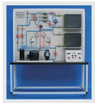
KR-115 is designed to learn the theory of Heat Transfer in refrigeration engineering. With proper setup, KR-115 can be emulated as a Refrigeration or Heat Pump system. All system components are mounted on the front panel so students can directly observe, touch the components, and hear the noise produced by the components while it is running under either Refrigeration or Heat Pump cycle.
